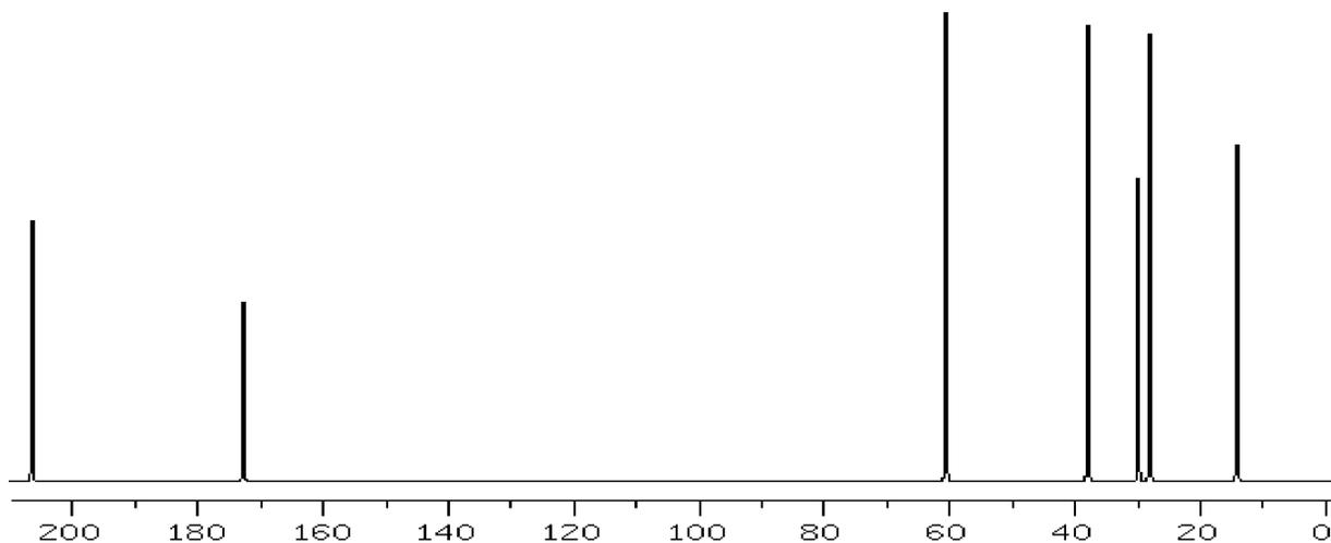
**Figure 5:**  $^{13}\text{C}$  NMR spectrum of ethyl levulinate (**4**)
